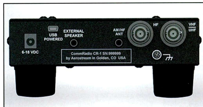
Photo C. The rear panel features jacks for connecting external antennas, speakers, and a USB 2 mini port.
