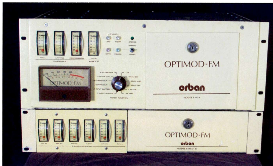
Photo C. In the '70s and '80s, the Orban Optimod — this one’s a model 8100 FM processor — ushered in a new era of modulation control for the broadcast industry, and even in today’s digital world, plenty of these “antique” analog Optimods are still on the air and are still sought after, serviced, and supported. ( Courtesy of Bohn Broadcast Services, Chelsea, Alabama )
