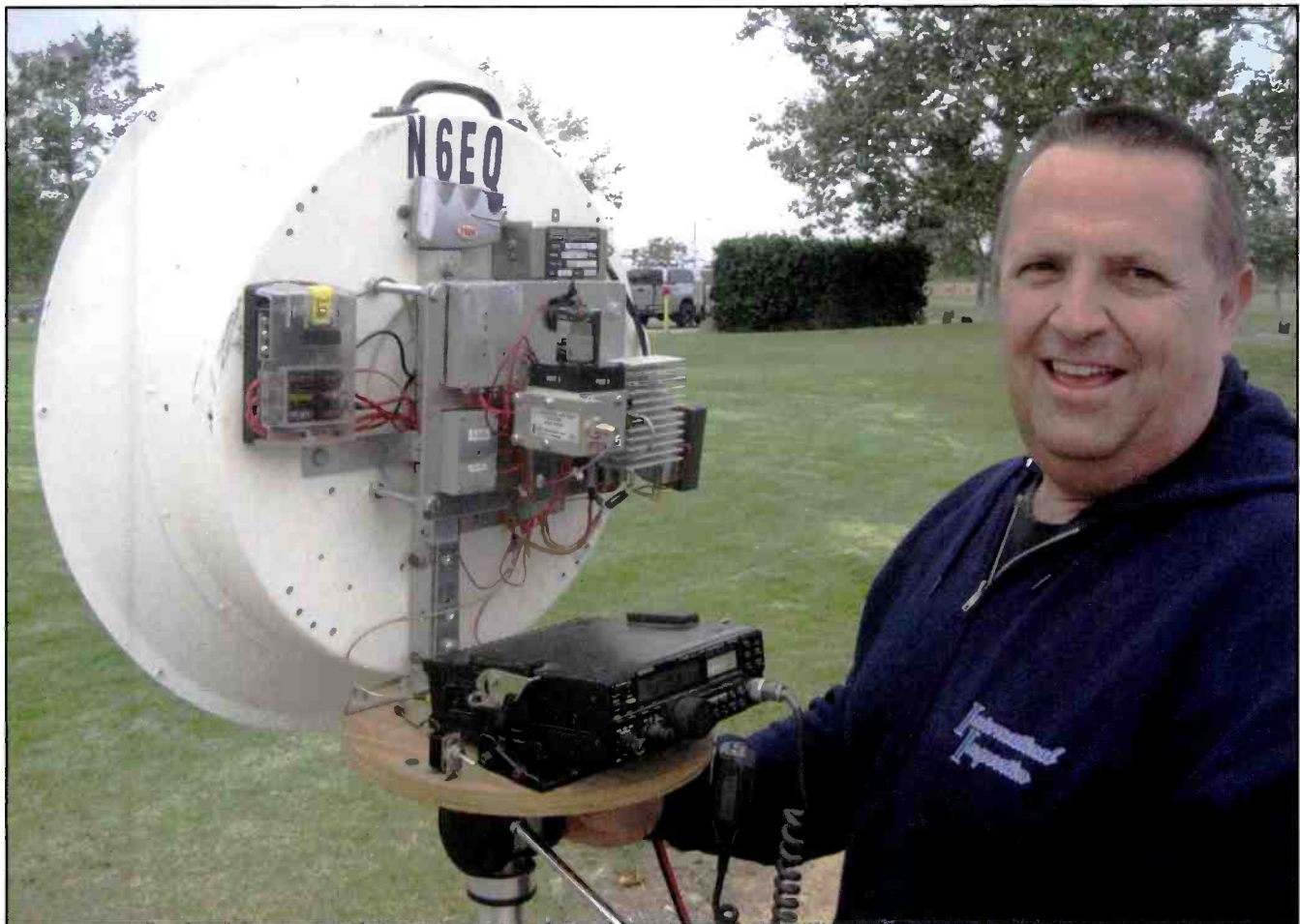
Photo C. Charles Olive, N6EQ, of Oak Hills, California, works microwave using a Kenwood transceiver and X-band transverter. It's a popular configuration for 10,000 MHz.
