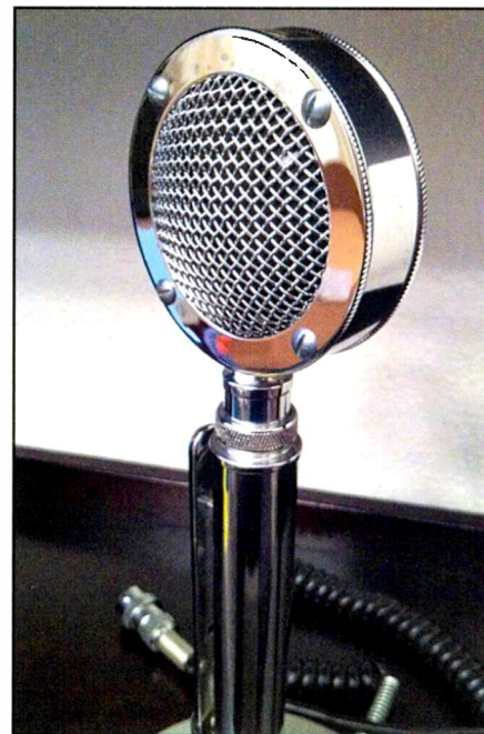
Photo B. “The venerable Drake transmitter had a classic Astatic D-104 crystal microphone,” KPCØZZZ writes, “and I was surprised that it sounded so good on the tube-powered Drake, but not very good at all on my solid-state Ten-Tec transceiver.” ( Internet screen grab < http://bit.ly/18ajs13 > )
